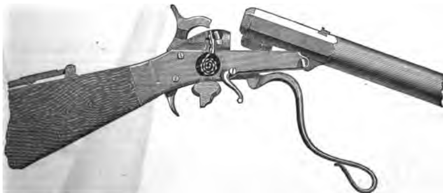
MAYNARD RIFLE.—Fig. 2. Showing Rifle in position to receive the cartridge, and with the magazine also opened, showing the primer.
